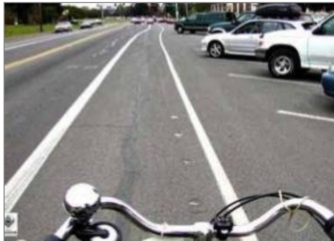
‘Back-in’ diagonal parking is safer for cyclists than ‘head-in’ diagonal parking due to drivers’ visibility as they exit the parking spot.
