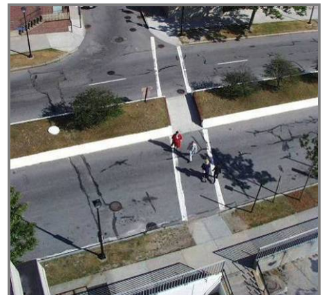
Median refuge islands break up a crossing and allow pedestrians to cross one side of a street at a time.
