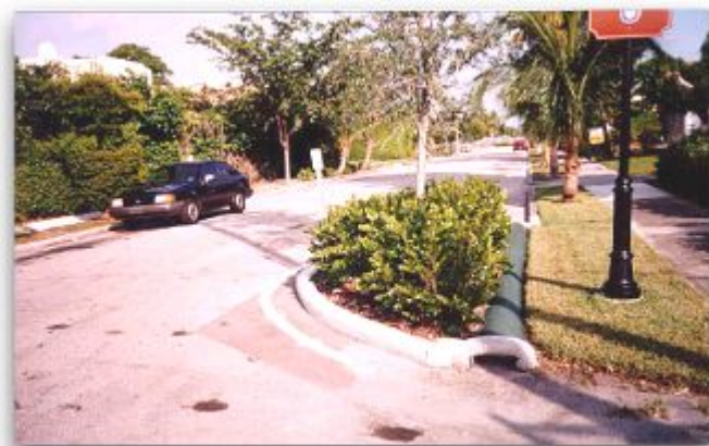
Illustration of a Chicane
