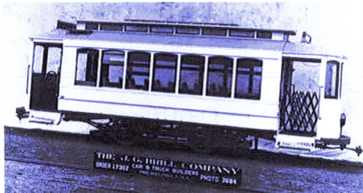
TEAK WOOD CAR OF BRILL SEMI-CONVERTIBLE TYPE. MOUNTED ON BRILL NO. 27-G1 TRUCKS.
