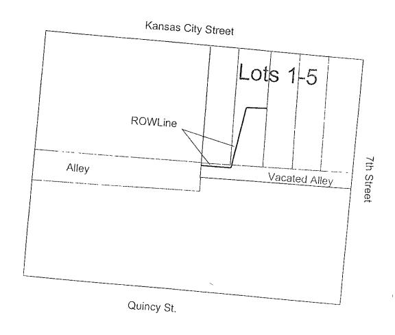
NOTE. The Centerline of the power line as constructed is the Center of the easement
