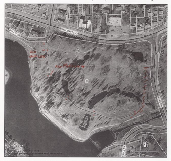
Remove for result PW013106-30 - Install 50' class A W-beam GR Resit 75 GR 12,5' Double class A W-beam GR By: Ched Hits JH Hilt Engineering INC. - The resett rail exisxing class Richibean GR (28 Ruse) (water) K 12.5 -> X - NO POST LETE. \* - Double class A"W-beam (12 gauge) This is done to span the 12.5ft distance and keep the system strength.
