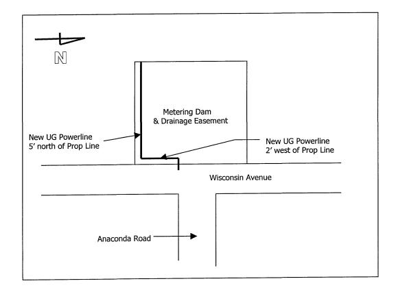
NOTE: The centerline of the powerline as constructed is the center line of the easement.
