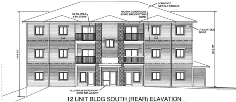
12 UNIT BLDG SOUTH (REAR) ELAVATION SCALE: 1/8" = 1'-0"
