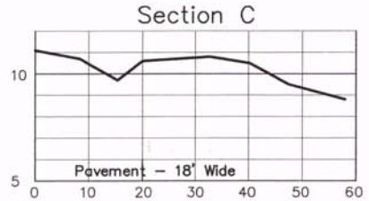
Cross Sections @ 1"=20' Horizontal - 1"=5' Vertical
