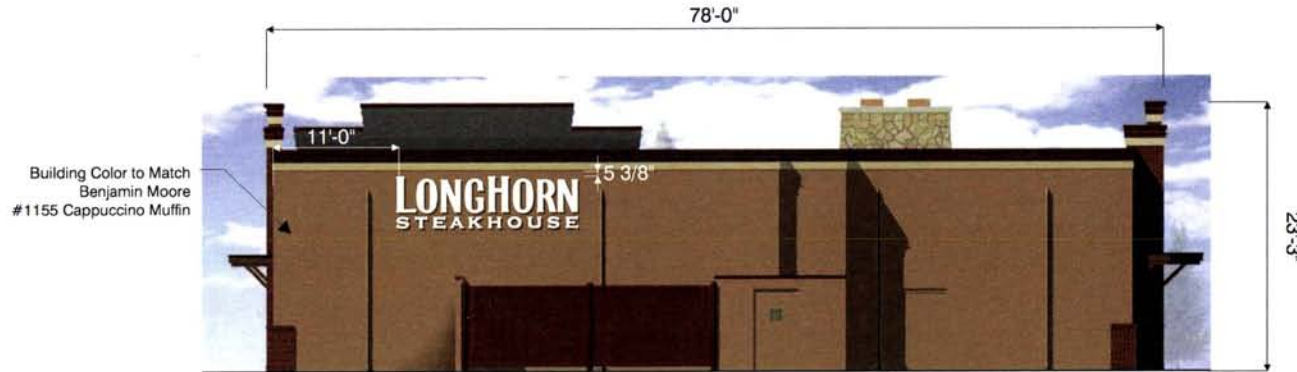
Measurements based on architectural plans provided. Measurements to be field verified. Red LED illuminated band to be mounted to cornice.
