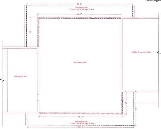
Safety Fence / Erosion Layout
