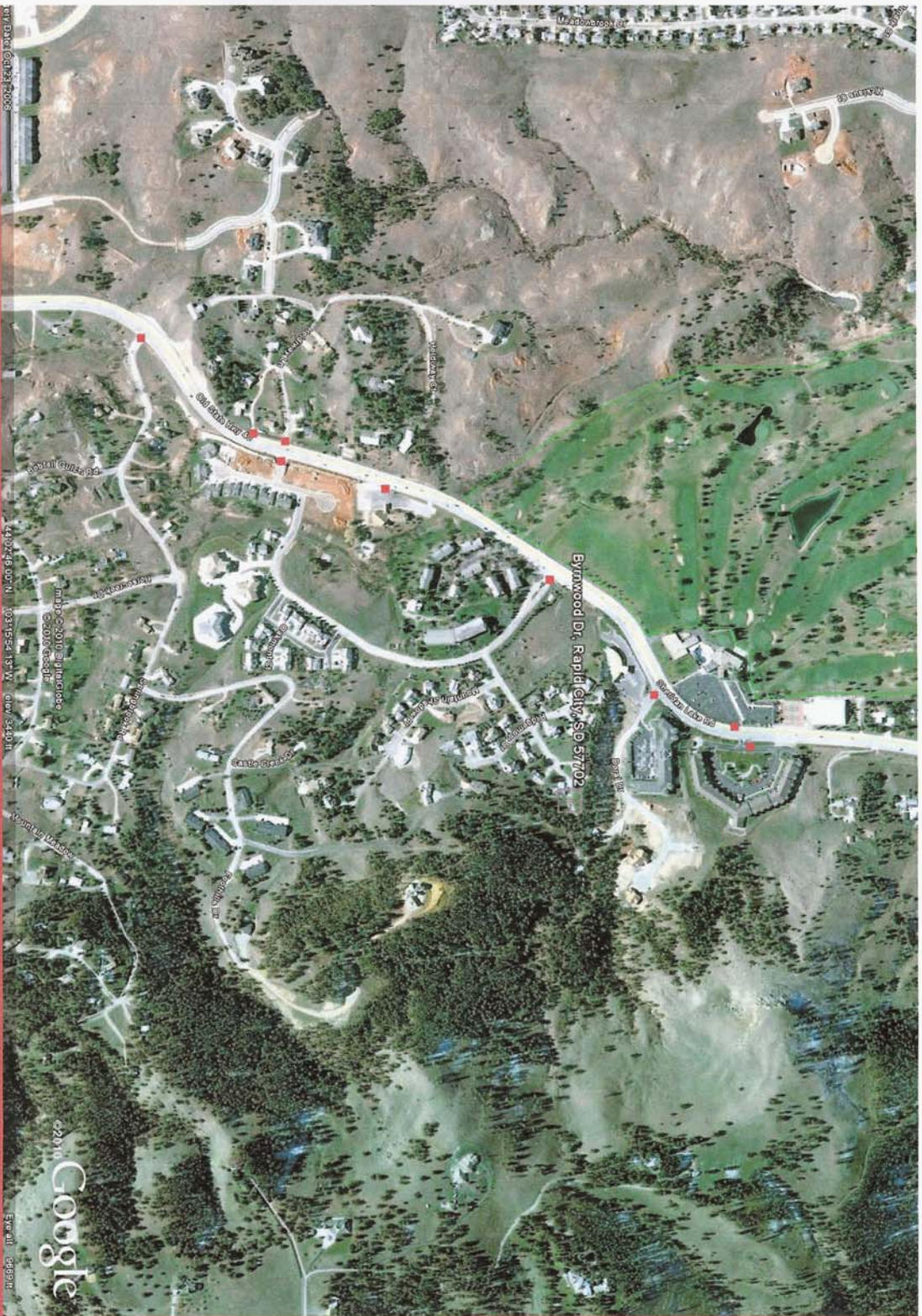
Semi-Blind Access Points Exiting On To Sheridan Lake Road, Resulting From “S” Curves and Gradient Changes.
