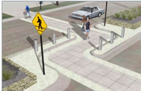
Right: Pedestrian Crossing. Connecting Wilson Park to the neighborhood towards the east is a midblock crossing. This type of crossing would be typical at various points along this segment of the corridor.
