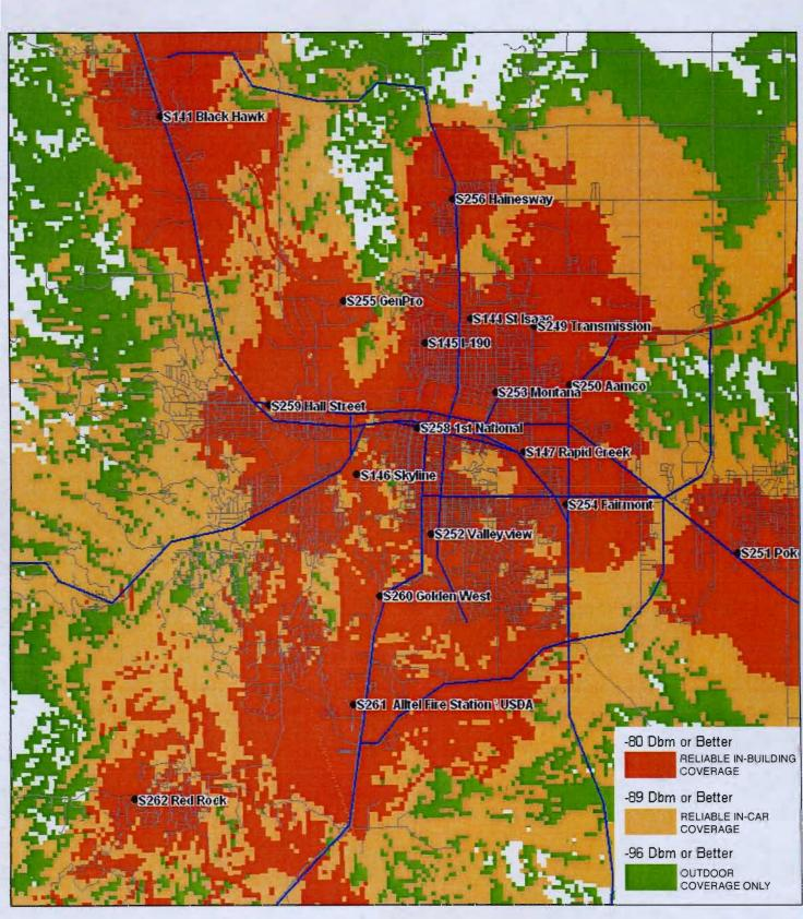
This RF coverage plot is based on an open rural topographical model. Coverage levels are predicted and are not a guarantee of actual or operational coverage.
