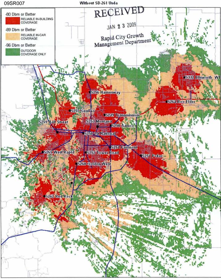
This RF coverage plot is based on an open rural topographical model. Coverage levels are predicted and are not a guarantee of actual or operational coverage.
