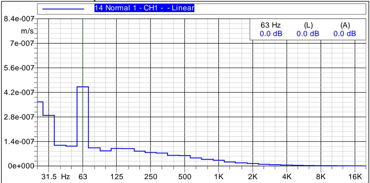
This figure shows that the maximum velocity occurred at 63 Hz. There are two large frequency spikes that appear on this graph – the first, a multi-frequency spike, centered at the octave band center of 25 Hz, the second at the octave band center of 63Hz.
