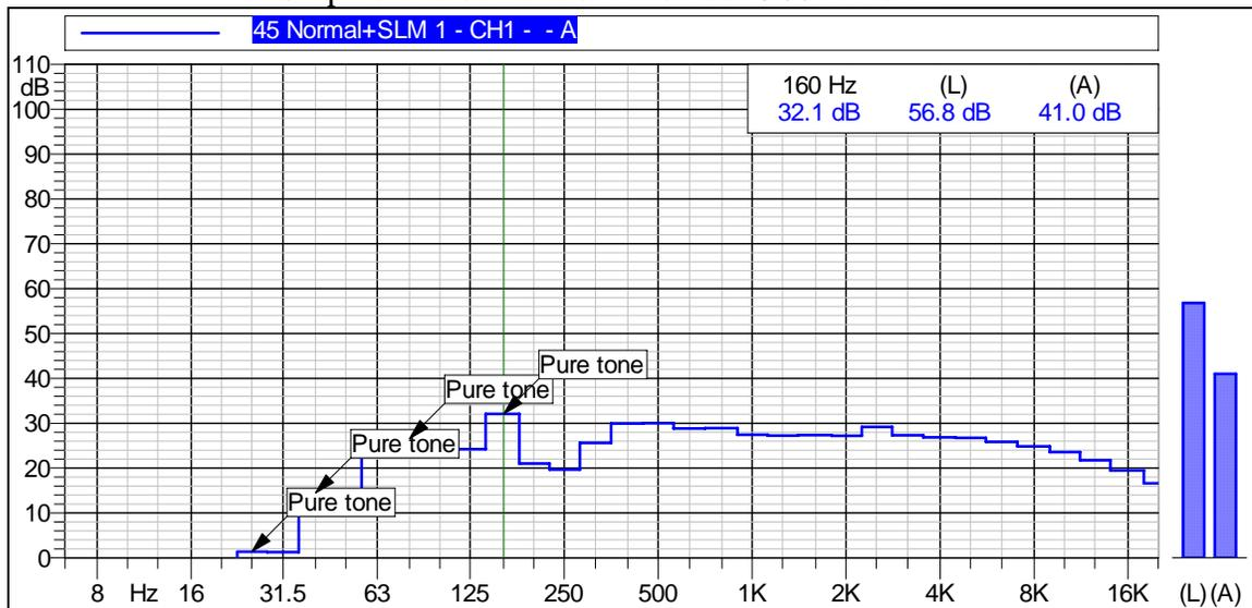
This figure shows that the Leq was 41 dBA and that the maximum sound pressure level of 32.1 dBA was measured at 160 Hz. Four pure tones appear on this graph – at 25, 40, 80, and 160 Hz. In the absence of background noises that can mask these tones, the tones may be considered annoying to some people. Pure tones at levels below 30 dBA may not be audible to the average person, particularly at frequencies below 80 Hz.
