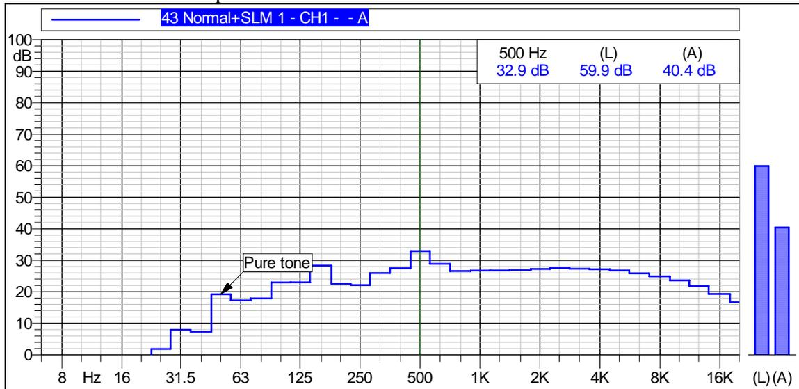
This figure shows that the Leq was 40 dBA and that the maximum sound pressure level of 32.9 dBA was measured at 500 Hz. A pure tone appears on this graph at 50 Hz though there is a peak at the 160 Hz octave band center. In the absence of background noises that can mask these tones, the tones may be considered annoying to some people. Pure tones at levels below 30 dBA may not be audible to the average person, particularly at frequencies below 80 Hz.
