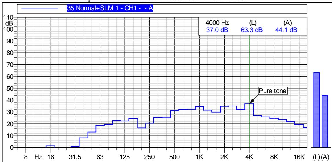
This figure shows that the Leq was 41 dBA and that the maximum sound pressure level of 37 dBA was measured at 4000 Hz. A pure tone appears on this graph, at 4000 Hz. In the absence of background noises that can mask this tone, the tone may be considered annoying to some people. Pure tones at levels below 30 dBA may not be audible to the average person, particularly at frequencies below 80 Hz.
