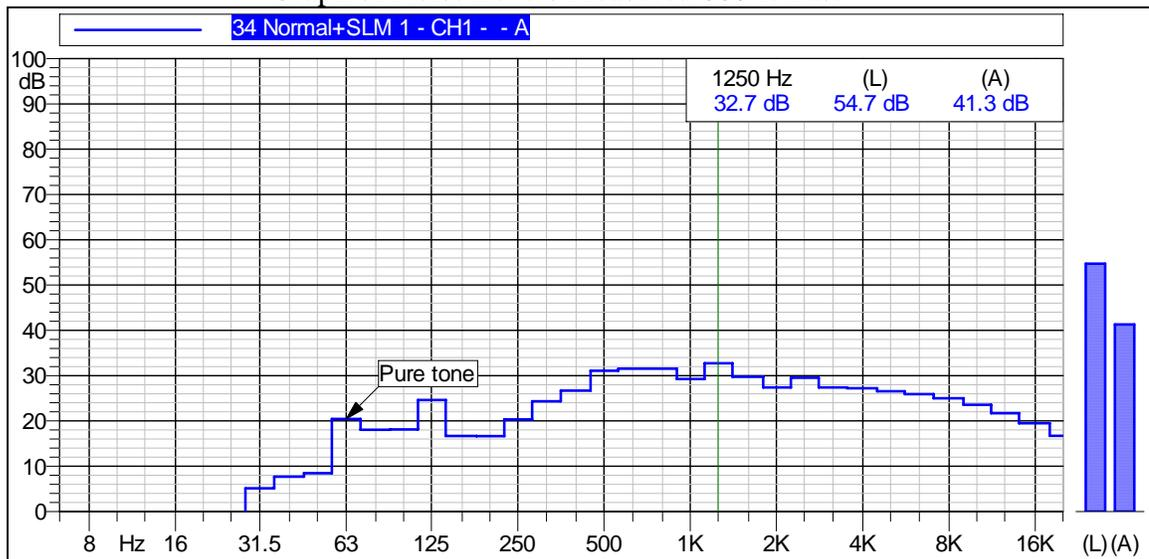
This figure shows that the Leq was 41 dBA and that the maximum sound pressure level of 32.7 dBA was measured at 1250 Hz. A pure tone appears on this graph, at 63 Hz though there is a peak at the 125 Hz octave band center. In the absence of background noises that can mask these tones, the tones may be considered annoying to some people. Pure tones at levels below 30 dBA may not be audible to the average person, particularly at frequencies below 80 Hz.
