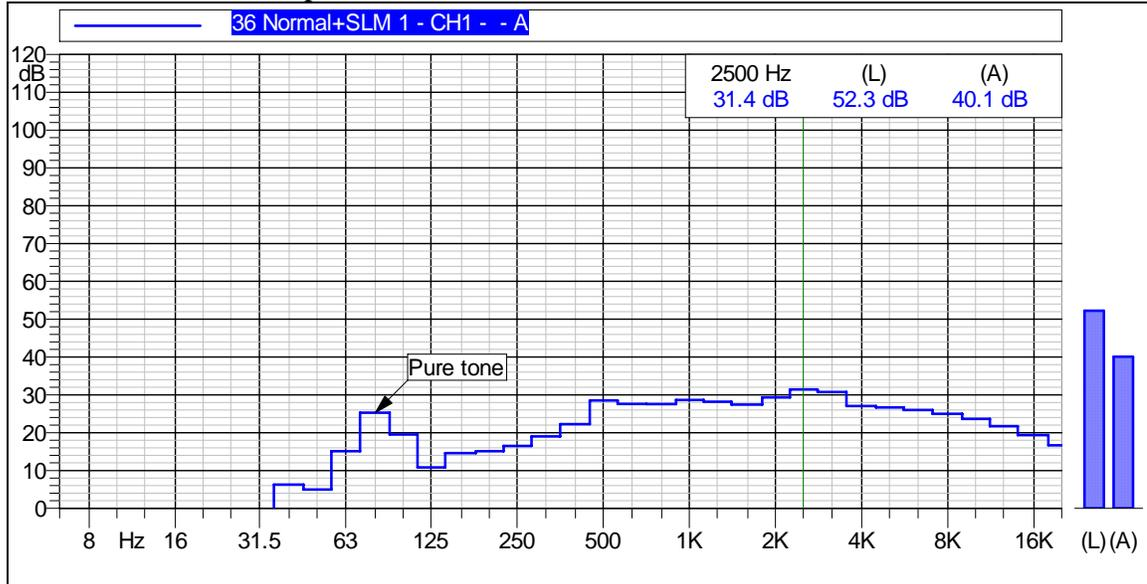
This figure shows that the Leq was 41 dBA and that the maximum sound pressure level of 31.4 dBA was measured at 2500 Hz. A pure tone appears on this graph at 80 Hz. In the absence of background noises that can mask this tone, the tone may be considered annoying to some people. Pure tones at levels below 30 dBA may not be audible to the average person, particularly at frequencies below 80 Hz.
