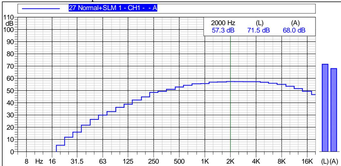
This figure shows that the Leq was 68 dBA and that the maximum sound pressure level of 57.3 dBA was measured at 2000 Hz.. No pure tones appear on this graph.
