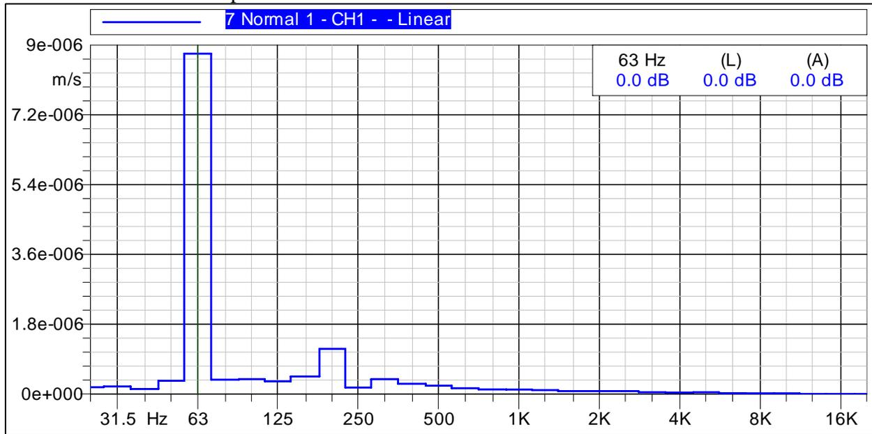
This figure shows that the maximum velocity occurred at 63 Hz. There is one large and one small frequency spike that appear on this graph – the first at the octave band center of 63 Hz, the second at 100 Hz.
