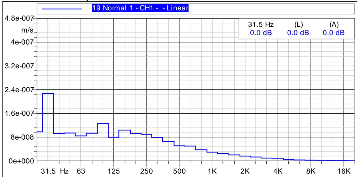
This figure shows that the maximum velocity occurred at 31.5 Hz. There is one large and one small frequency spikes that appear on this graph – the first at the octave band center of 31.5 Hz, the second at 100Hz.
