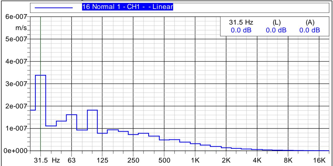
This figure shows that the maximum velocity occurred at 31.5 Hz. There is one large and one small frequency spike that appear on this graph – the first at the octave band center of 31.5 Hz, the second at 100 Hz.
