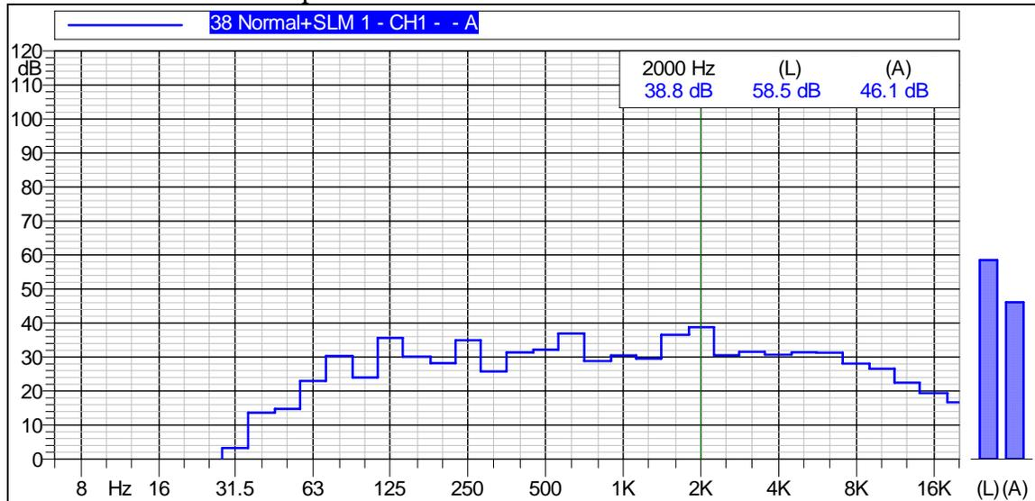
This figure shows that the Leq was 46 dBA and that the maximum sound pressure level of 38.8 dBA was measured at 2000 Hz. Pure tones do not appear on this graph. However, there are elevated levels at 80, 125, 250, 630 Hz. In the absence of background noises that can mask these tones, the tones may be considered annoying to some people.
