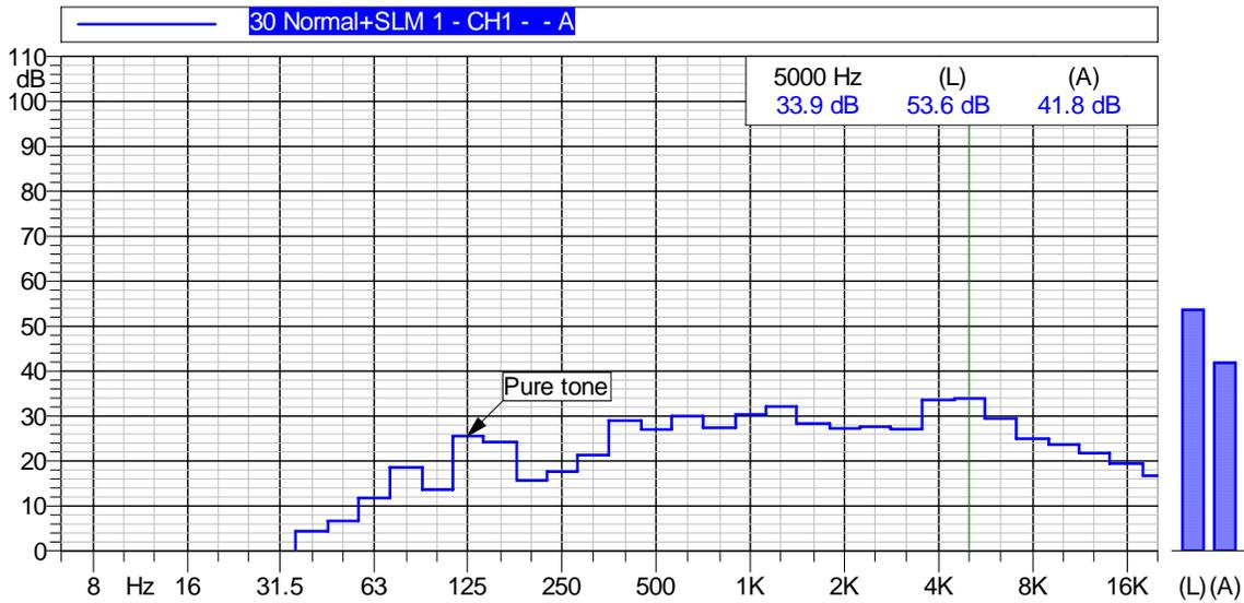
This figure shows that the Leq was 42 dBA and that the maximum sound pressure level of 33.9 dBA was measured at 5000 Hz. The data processing software identified a pure tone at 125 Hz. There is also smaller peak at the 80 Hz octave band center. In the absence of background noises that can mask these tones, the tones may be considered annoying to some people. Pure tones at levels below 30 dBA may not be audible to the average person, particularly at frequencies below 80 Hz.
