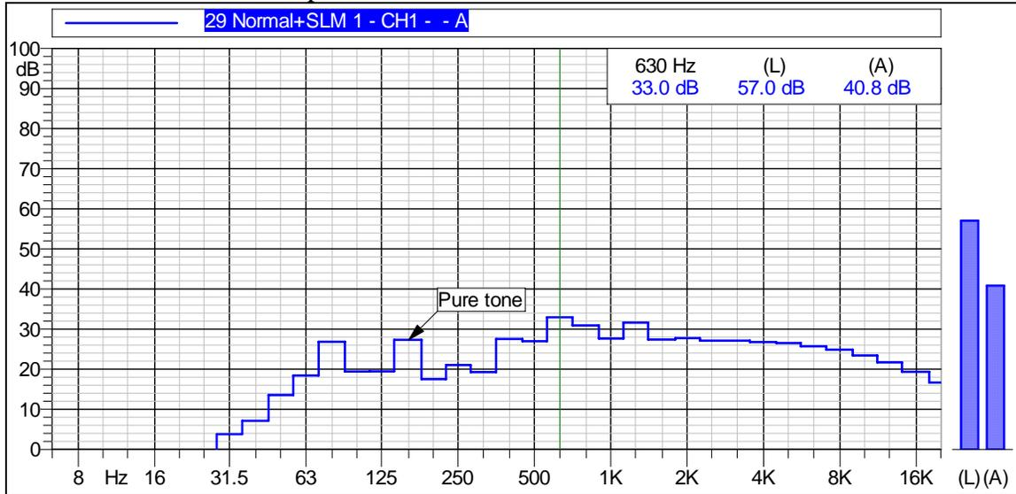
This figure shows that the Leq was 40.8 dBA and that the maximum sound pressure level of 33 dBA was measured at 630 Hz. A pure tone appears on this graph, at 160 Hz. There is also a peak at the 80 Hz octave band center. In the absence of background noises that can mask these tones, the tone may be considered annoying to some people. Pure tones at levels below 30 dBA may not be audible to the average person, particularly at frequencies below 80 Hz.
