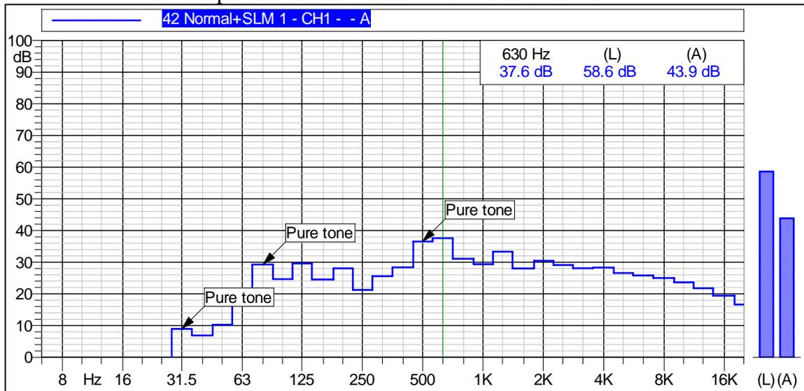
This figure shows that the Leq was 43.9 dBA and that the maximum sound pressure level of 37.6 dBA was measured at 630 Hz. Pure tones appear on this graph, at 31.5, 80, and 800 Hz. There are also peaks at 125, 200, and 1250 Hz octave band centers. In the absence of background noises that can mask these tones, the tones may be considered annoying to some people. Pure tones at levels below 30 dBA may not be audible to the average person, particularly at frequencies below 80 Hz.
