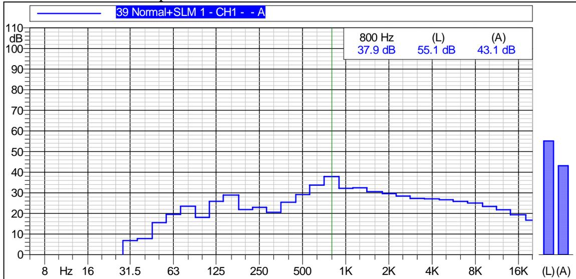
This figure shows that the Leq was 43.1 dBA and that the maximum sound pressure level of 37.9 dBA was measured at 800 Hz. No pure tones appear on this graph. However there are peaks at 80, between 125 and 160, and at 800 Hz. In the absence of background noises that can mask these tones, the tones may be considered annoying to some people. Pure tones at levels below 30 dBA may not be audible to the average person, particularly at frequencies below 80 Hz.
