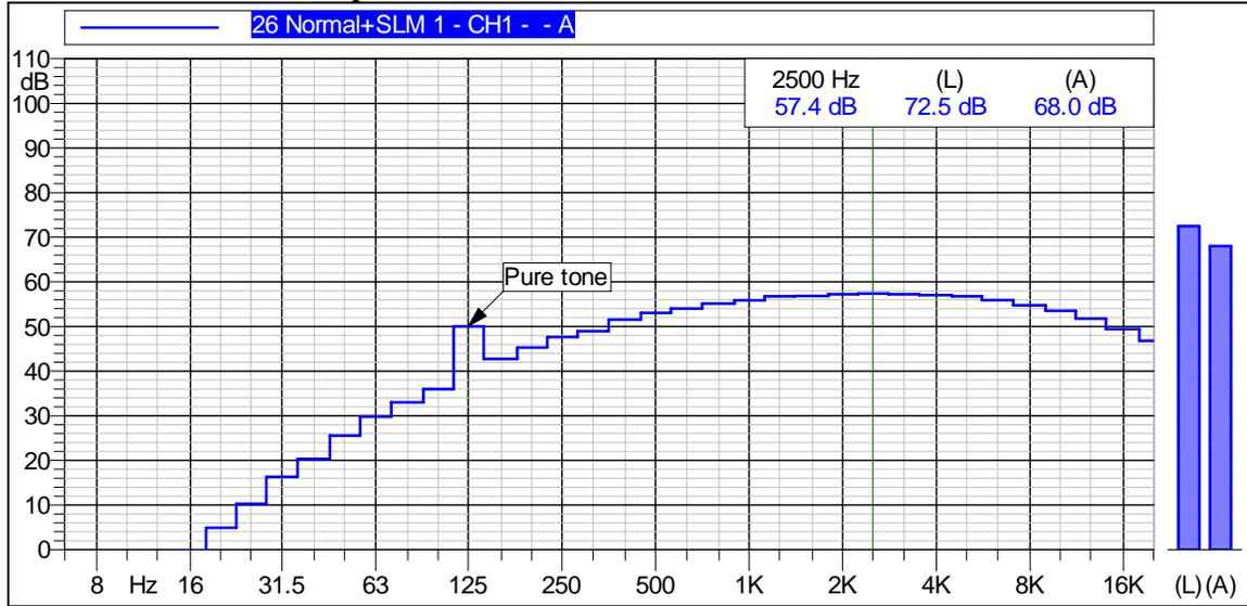
This figure shows that the Leq was 68 dBA and that the maximum sound pressure level of 57.4 dBA was measured at 2500 Hz. A pure tone appears on this graph, at 125 Hz. In the absence of background noises that can mask these tones, the tone may be considered annoying to some people.
