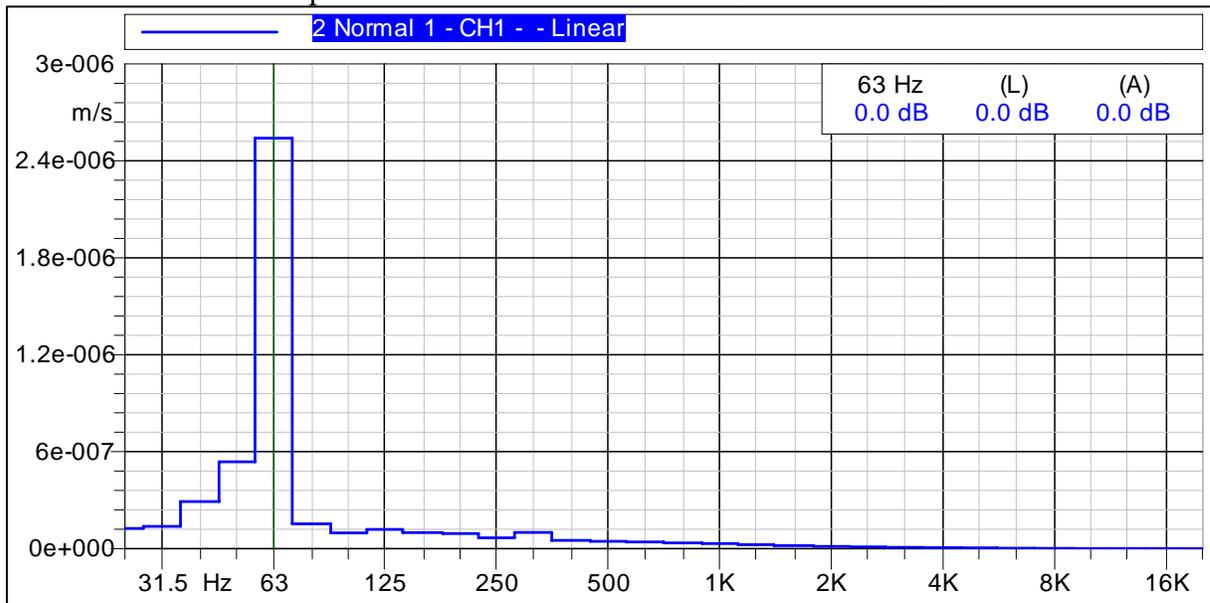
This figure shows that the maximum velocity occurred at 63 Hz. There is one frequency spike that appears on this graph – at the octave band center of 63 Hz.
