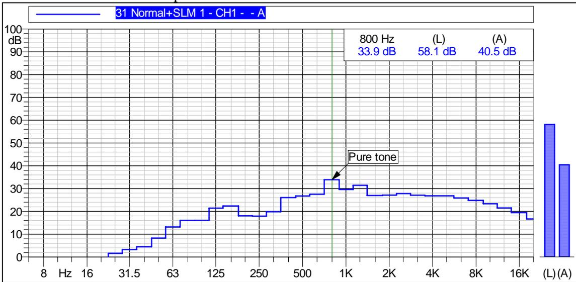
This figure shows that the Leq was 41 dBA and that the maximum sound pressure level of 33.9 dBA was measured at 800 Hz. A pure tone appears on this graph, at 800 Hz.
