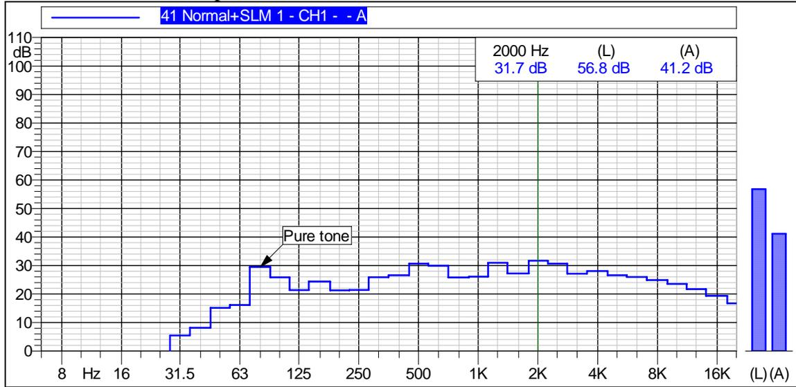
This figure shows that the Leq was 41.2 dBA and that the maximum sound pressure level of 31.7 BA was measured at 2000 Hz. A pure tone appears on this graph, at 80 Hz. In the absence of background noises that can mask these tones, the tones may be considered annoying to some people. Pure tones at levels below 30 dBA may not be audible to the average person, particularly at frequencies below 80 Hz.
