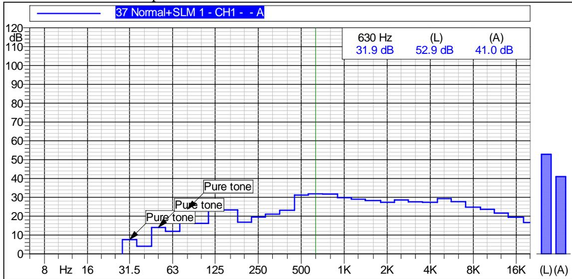
This figure shows that the Leq was 41 dBA and that the maximum sound pressure level of 31.9 dBA was measured at 630 Hz. Pure tones appear on this graph, at 31.5, 50, and 80 Hz though there are peaks at the 125 and 160 Hz octave band centers. In the absence of background noises that can mask these tones, the tones may be considered annoying to some people. Pure tones at levels below 30 dBA may not be audible to the average person, particularly at frequencies below 80 Hz.
