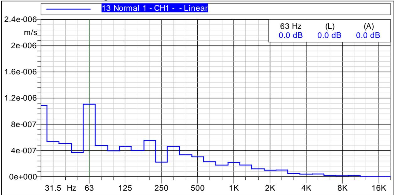
This figure shows that the maximum velocity occurred at 63 Hz. There are two large frequency spikes that appear on this graph – the first at the octave band center of 25 Hz, the second at the octave band center of 63Hz.
