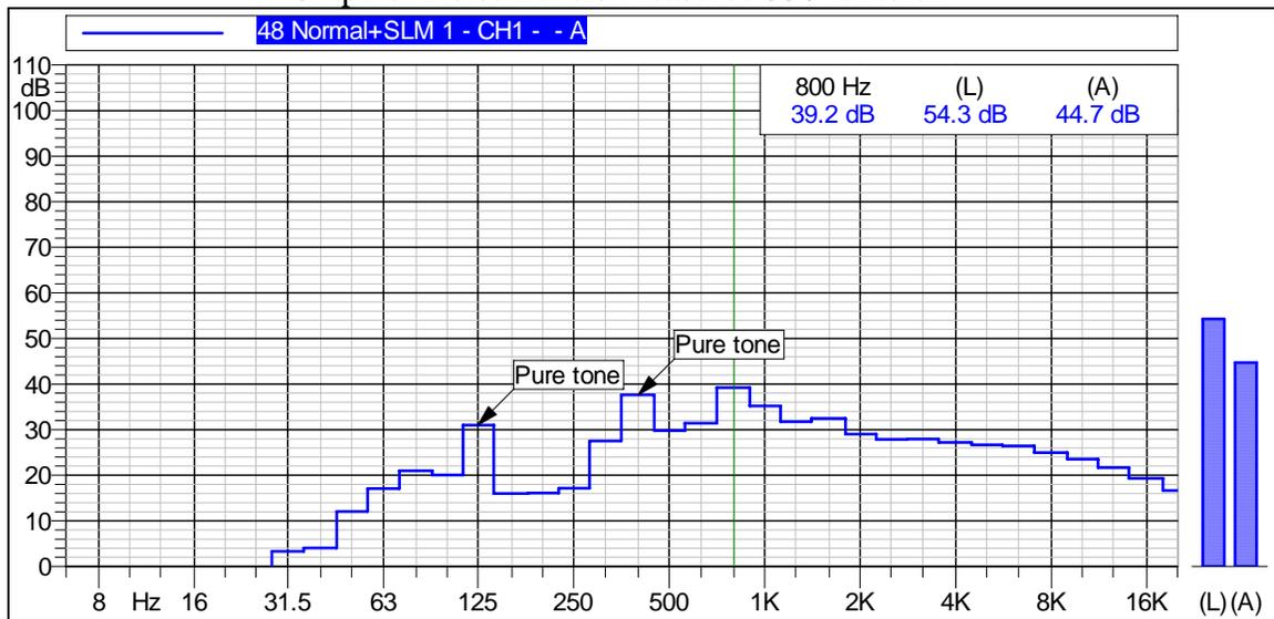
This figure shows that the Leq was 44.7 dBA and that the maximum sound pressure level of 39.2 dBA was measured at 800 Hz. Two pure tones appear on this graph – first at the octave band center at 125 Hz and again at 400 Hz. There also appears to be something close to a pure tone at 800 Hz. In the absence of background noises that can mask these tones, the tones may be considered annoying to some people.
