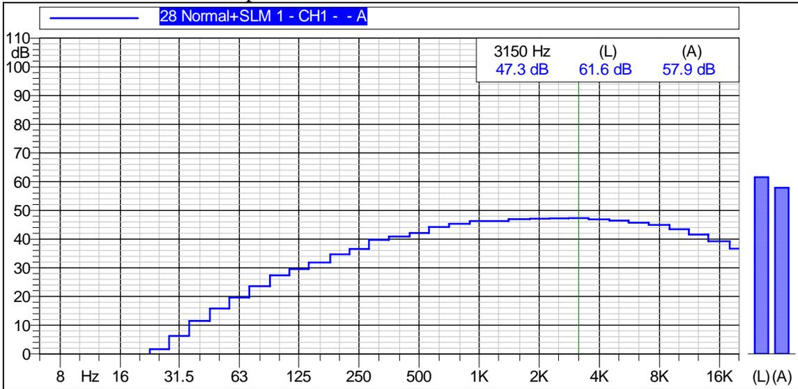
This figure shows that the Leq was 57.9 dBA and that the maximum sound pressure level of 47.3 dBA was measured at 3150 Hz. No pure tones appear on this graph.
