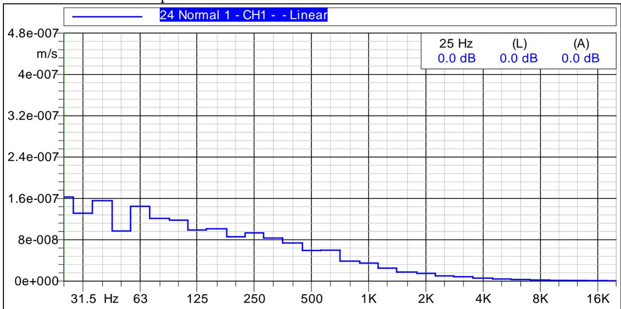
This figure shows that the maximum velocity occurred at 25 Hz. There are no frequency spikes that appear on this graph.
