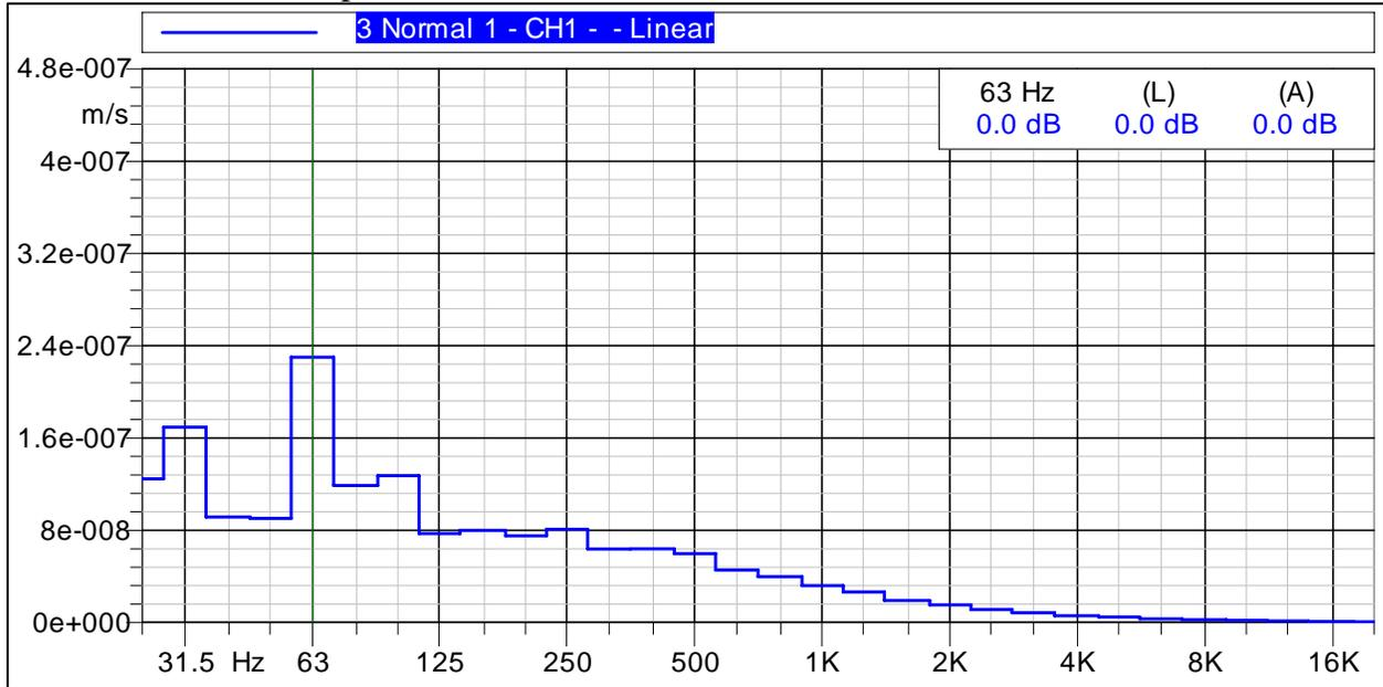
This figure shows that the maximum velocity occurred at 63 Hz. There is one large and one small frequency spike that appear on this graph – the first at the octave band center of 63 Hz, the second at the octave band center of 31.5Hz.
