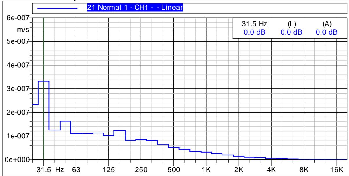
This figure shows that the maximum velocity occurred at 31.5 Hz. There is one frequency spike that appears on this graph – at the octave band center of 31.5 Hz.
