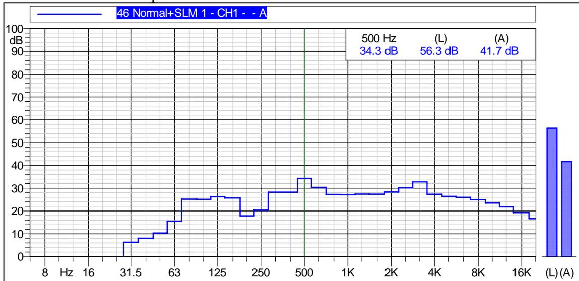
This figure shows that the Leq was 41.7 dBA and that the maximum sound pressure level of 34.3 dBA was measured at 500 Hz. No pure tones appear on this graph, though there is a peak at the 500 Hz octave band center. In the absence of background noises that can mask these tones, the tones may be considered annoying to some people.
