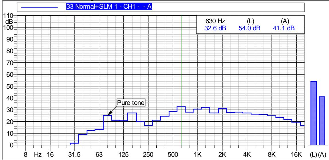
This figure shows that the Leq was 41 dBA and that the maximum sound pressure level of 32.6 dBA was measured at 630 Hz. A pure tone appears on this graph, at 80 Hz though there is a peak at the 160 Hz octave band center. In the absence of background noises that can mask these tones, the tones may be considered annoying to some people. Pure tones at levels below 30 dBA may not be audible to the average person, particularly at frequencies below 80 Hz.
