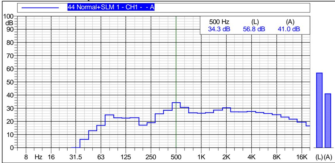
This figure shows that the Leq was 41 dBA and that the maximum sound pressure level of 34.3 dBA was measured at 500 Hz. No pure tones appear on this graph, though there is a peak at the 500 Hz octave band center. In the absence of background noises that can mask these tones, the tones may be considered annoying to some people
