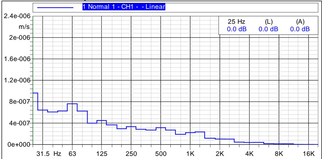
This figure shows that the maximum velocity occurred at 25 Hz. There is one frequency spike that appears on this graph – at 25 Hz.
