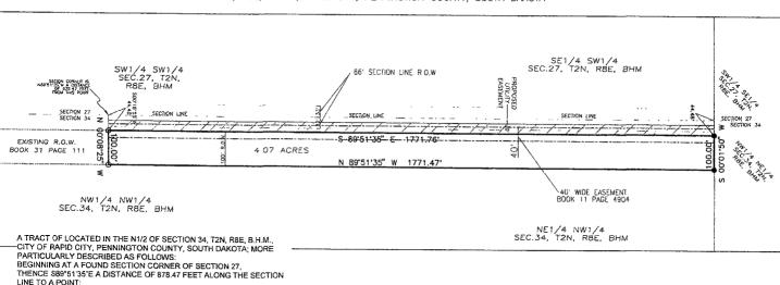
THENCE \$00°18'55"W A DISTANCE OF 44.48 FEET TO THE TRUE POINT OF BEGINNING AT A FOUND REBAR AND CAP STAMPED "ARLETH AND ASSOCIATES LS 3977" THIS BEING THE TRUE POINT OF BEGINNING: THENCE S89°51'35"E A DISTANCE OF 1771.76 FEET TO A ANGLE POINT.
