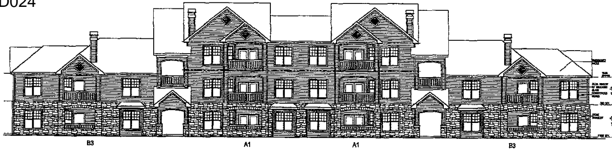
BLDG. TYPE I - A1/B3 SCALE: 1/8"=1'-0" FRONT ELEVATION
