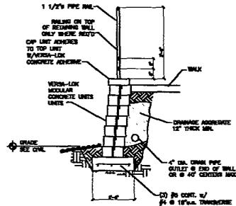
TYPICAL SECTION—UNREINFORCED RETAINING WALL
