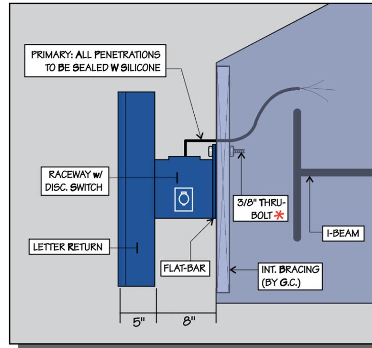
\* NOTE : IF THIS AREA IS NOT ACCESSIBLE, A 3/8" TOGGLE MUST BE USED (THRU METAL FASCIA & BACKING).
