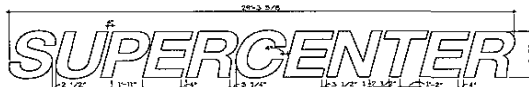
HELVECTICA MEDIUM WITH 1/8" SLANT SOLID MOUNT PLASTIC LETTERS NOTE: SUPERCENTER STOREFRONT SIGNAGE ONLY REG. LETTERS
