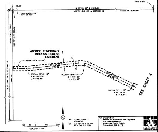
THE BASIS OF BEARING FOR THIS PLAT IS N89° 53'58"E ALONG THE NORTH LINE OF THE SW 1/4 OF SECTION 16 AS SHOWN HEREON.
