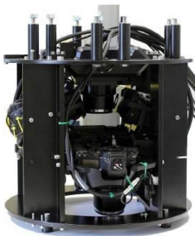
Panoramix Camera Array: The camera system is configured with four oblique cameras (mounted at 45 degrees) and one nadir facing camera.
