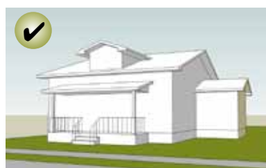
Small Side Addition: Set back behind the facade and remains subordinate.
