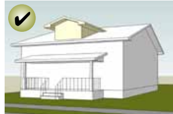
Small Gable Dormer: Addition is centered and located below the roof ridge, remains subordinate.
