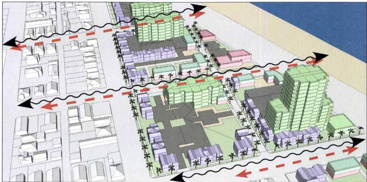
Sustainability design standards and guidelines help ensure that taller, higher density development in Galveston, Texas, considers view corridors and breezeways along the streets leading to established neighborhoods.
