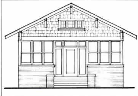
Existing Condition: Craftsman style house with an enclosed porch.
