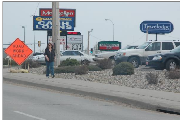
Figure 5. Curb-tight sidewalks on arterials can be an uncomfortable walking environment.
