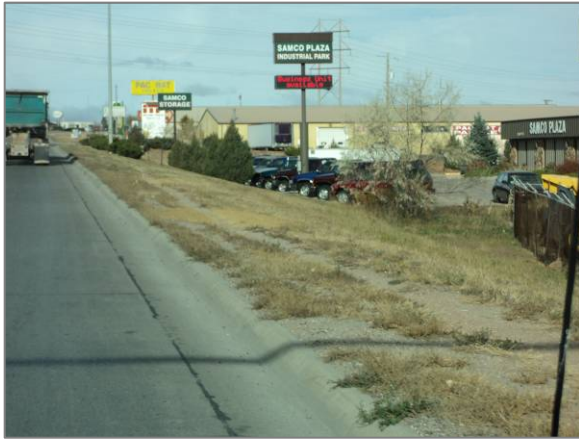
Figure 8. Frequent pedestrian use along Deadwood Avenue is evident by the worn “demand trail”, indicating a good location for a pedestrian facility investment.
