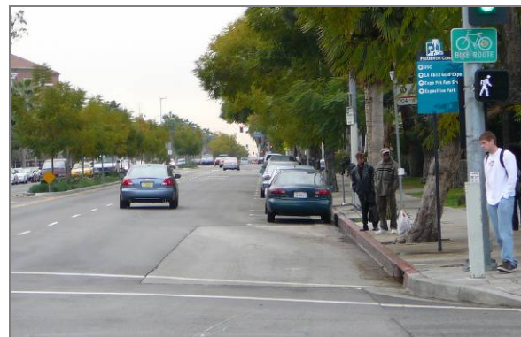
This bike route in Los Angeles provides a wide outside lane adjacent to on-street parking.
