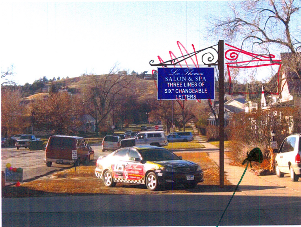
48" x 84" DF MDO East side (facing Mt. Rushmore Rd.) 18' x 6" pole Minimum 8' clearance
