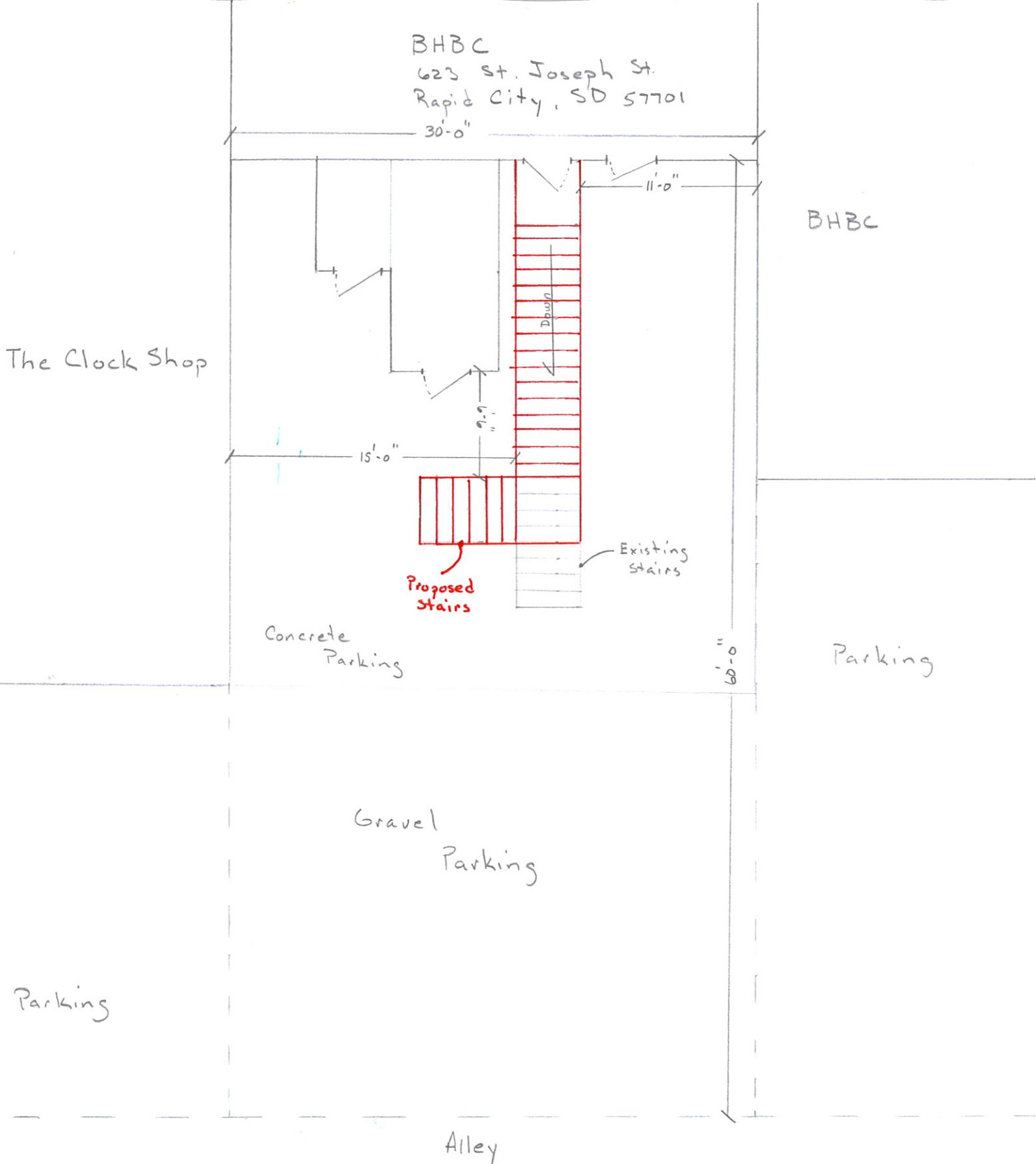
Remove and replace the existing set of stairs that go from the ground level to the second floor of our building. These stairs are used to exit the building in case of an emergency. The new set of stairs will be constructed of steel to replace the current wood framed stairs. Both the current stairs and the proposed stairs land on an existing concrete pad.
