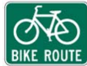
Bike Route signs are used to indicate the street is designated for bicycle use.
