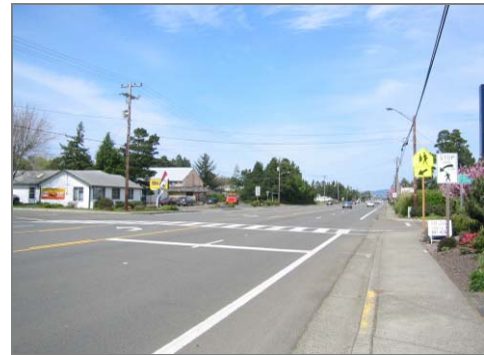
Advance stop bars alert motorists of pedestrians.
