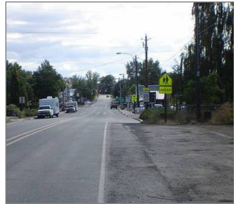
Roadway widening is preferred on roads lacking curbs, gutters and sidewalks.
