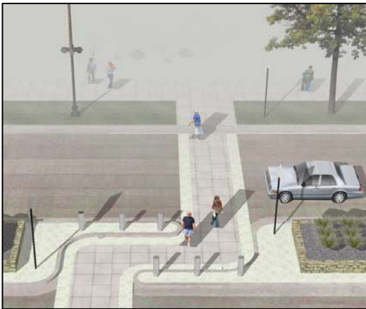
Figure 35. Mid-Block Pedestrian Crossing Concept.
