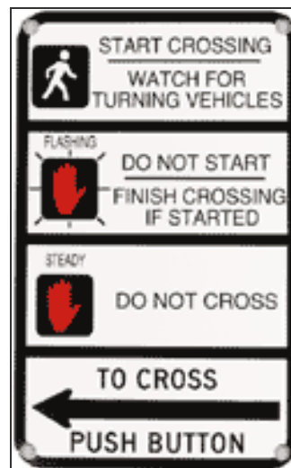
Pedestrian push buttons can be accompanied by informational signage.
