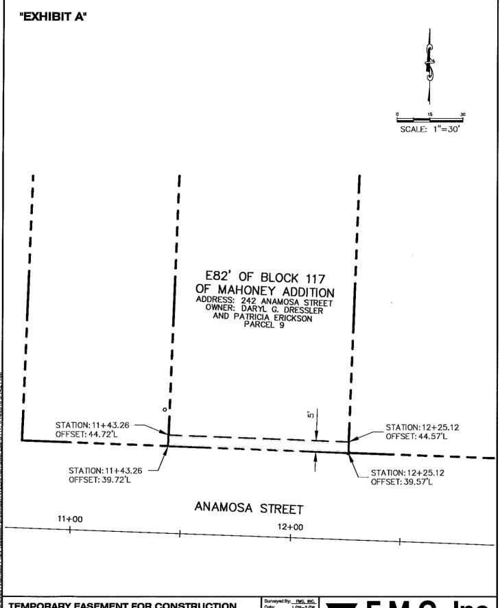
**TEMPORARY EASEMENT FOR CONSTRUCTION E82' OF BLOCK 117 OF MAHONEY ADDITION** SE 1/4, SEC. 25, T2N, R7E, BHM
