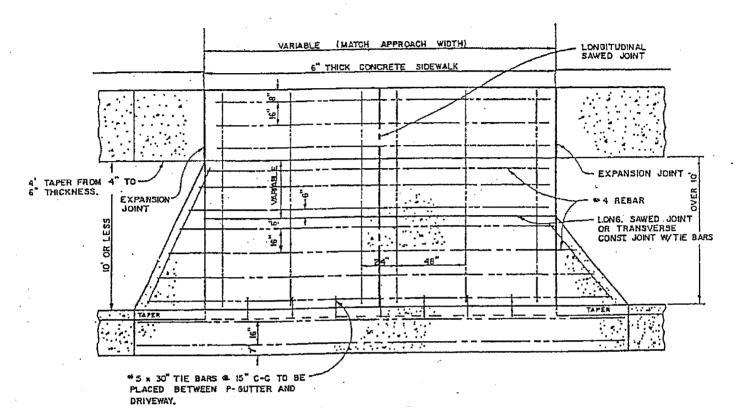
WHEN REMOVING EXISTING CURB AND GUTTER FOR NEW APPROACH CONSTRUCTION, AN EXPANSION JOINT SHALL BE CONSTRUCTED. (SEE JOINT DETAILS).
