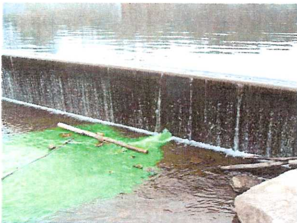
Photos 7 & 8 – March 2005, Midco Diving dye testing shows an extensive amount of dye exiting the underdrain pipe outlet at the base of the concrete apron downstream of the spillway.
