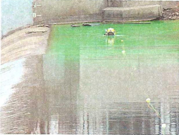
Photos 1 & 2 – March 2005, Midco Diving releasing the dye for seepage testing near the upstream sinkhole.
