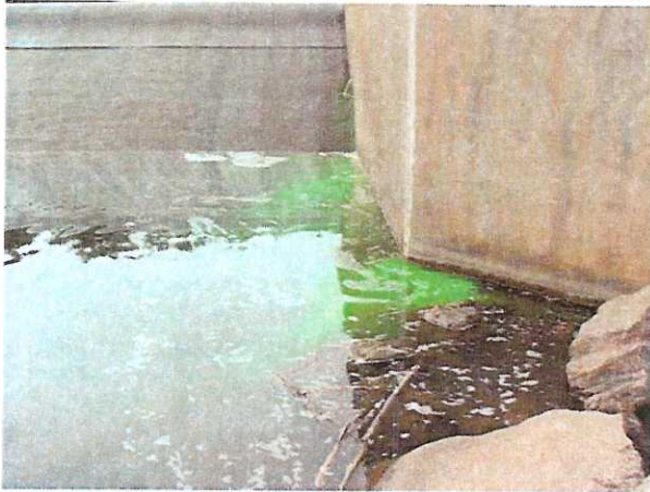
Photos 4 & 5 – March 2005, Midco Diving dye testing reveals plumes of dye emerging from the weep holes and areas along the spillway wing walls.
