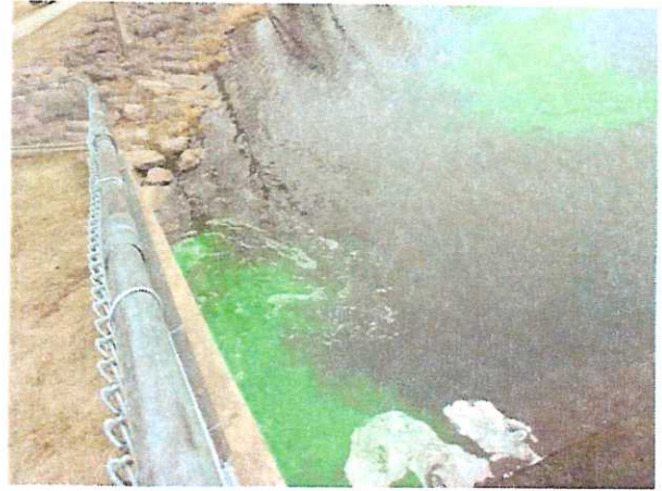
Photos 4 & 5 – March 2005, Midco Diving dye testing reveals plumes of dye emerging from the weep holes and areas along the spillway wing walls.
