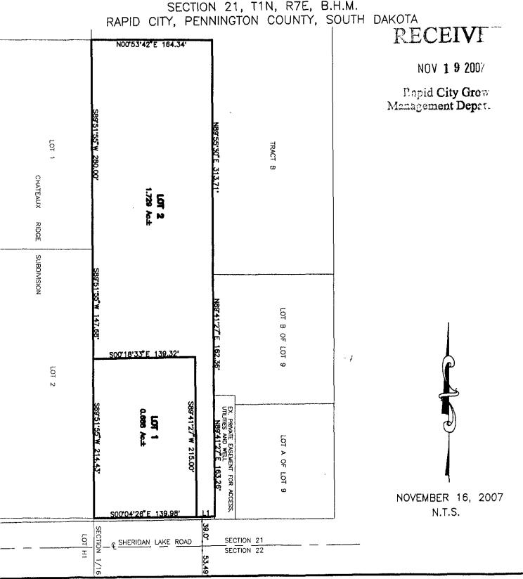
(Formerly Et of Lot 8 of Et of NEW less Lot H1 of Et of Lot 8 of Et of NEW all in Section 21, TIN, R7E, BMM) Located in NEk of NEk of Section 21, TIN, R7E, SHM, Rapid City, Pennington County, South Dakota LEGEND: Set 5/8" rebar with survey cap marked "HEALD SD 2199".
