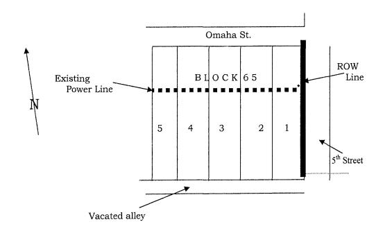
NOTE: The centerline of the powerline as constructed is the center line of the easement.
