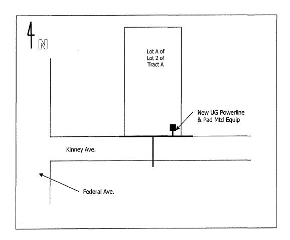
NOTE: The centerline of the powerline as constructed is the center line of the easement.
