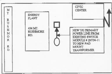
NOTE: The centerline of the powerline as constructed is the center line of the easement.
