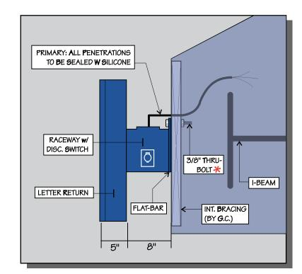
\*NOTE: IF THIS AREA IS NOT ACCESSIBLE, A 3/8" TOGGLE MUST BE USED (THRU METAL FASCIA & BACKING).
