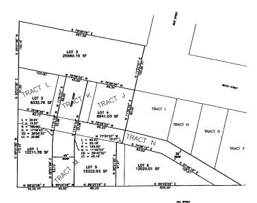
1. 8' WIDE UTILITY AND DRAINAGE EASEMENT ON EACH SIDE OF ALL FRONT, SIDE, AND REAR LOT LINES.
